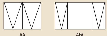
Awnings go to 1800 high as a single unit. As in Sliding and Double Hung, fixed lites can be fitted either horizontally or vertically to give a wide choice of sizes and designs.
